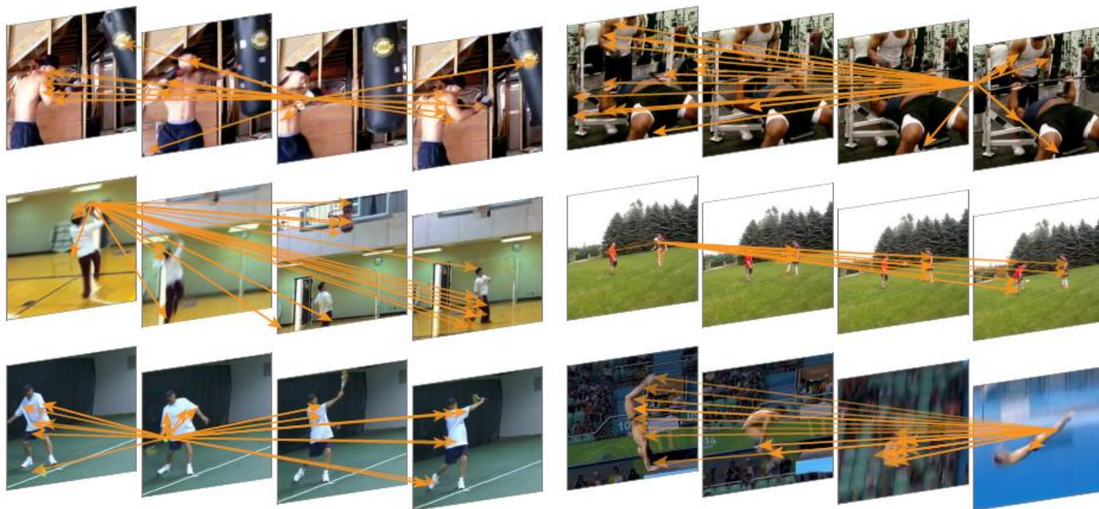
Figure 3. Examples of the behavior of a non-local block in res_3 computed by a 5-block non-local model trained on Kinetics. These examples are from held-out validation videos. The starting point of arrows represents one x_i , and the ending points represent x_j . The 20 highest weighted arrows for each x_i are visualized. The 4 frames are from a 32-frame input, shown with a stride of 8 frames. These visualizations show how the model finds related clues to support its prediction.
